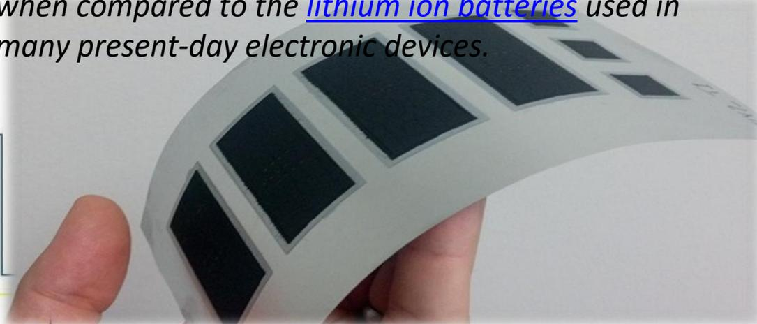
Specialized paper batteries are expected to act as power sources for any number of devices implanted in humans and animals, including [RFID](#) tags, drug-delivery systems and pacemakers. In theory, a capacitor introduced into an organism could be implanted fully dry and then be gradually exposed to bodily fluids over time to generate voltage.
