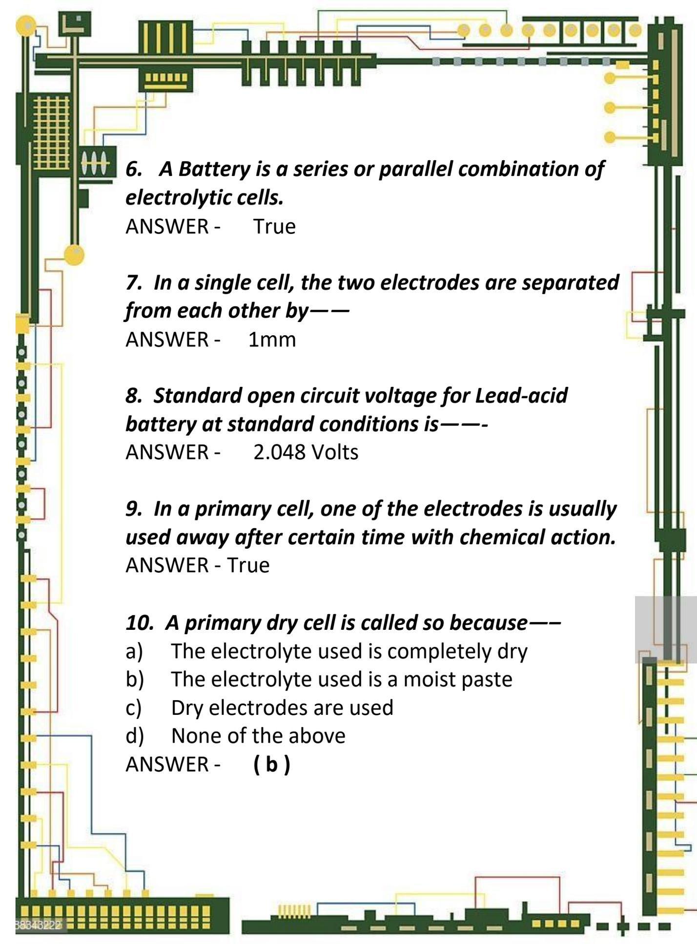
**6. A Battery is a series or parallel combination of electrolytic cells.**
